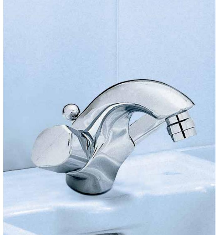
*Mono-block, dual-control, bidet fitting* with ceramic-disk, 1/4-turn cartridges and cast brass body. Includes directional ball-joint, handles and pop-up waste.
