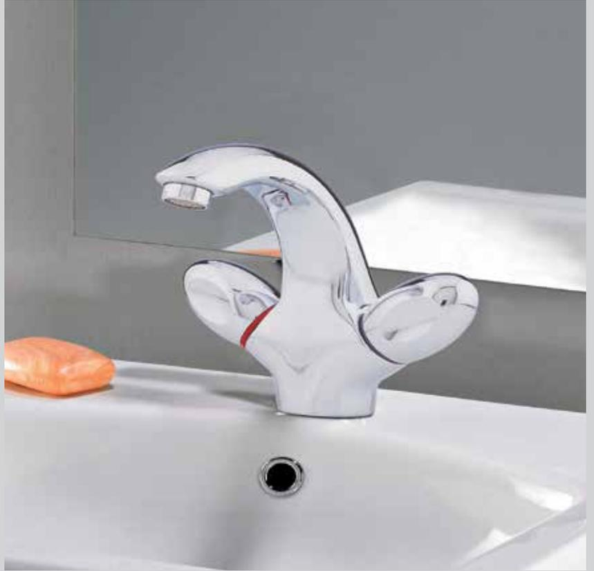
**Mono-block** dual-control, basin mixer, swivel spout with ceramic-disk, 1/4-turn cartridges and cast brass body with flexible-hose, supply connections. Includes handles and pop-up waste.
