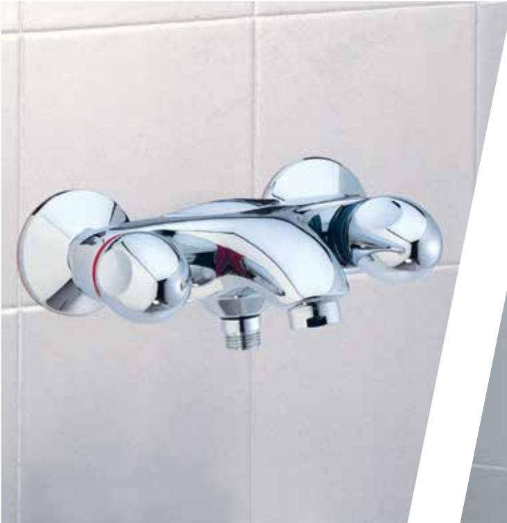
**Dual-control wall-exposed** bath & shower fitting with ceramic-disk, 1/4-turn cartridges and cast brass body. Includes handles.
