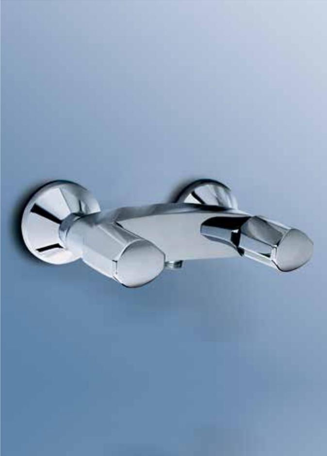
*Dual-control* wall-exposed, shower fitting with ceramic-disk, 1/4-turn cartridges and cast brass body. Includes handles.
