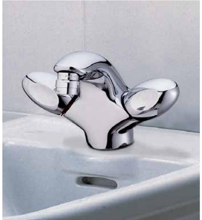
*Mono-block* dual-control, bidet fitting with ceramic-disk, 1/4-turn cartridges and cast brass body, Includes directional ball-joint, handles and pop-up waste.
