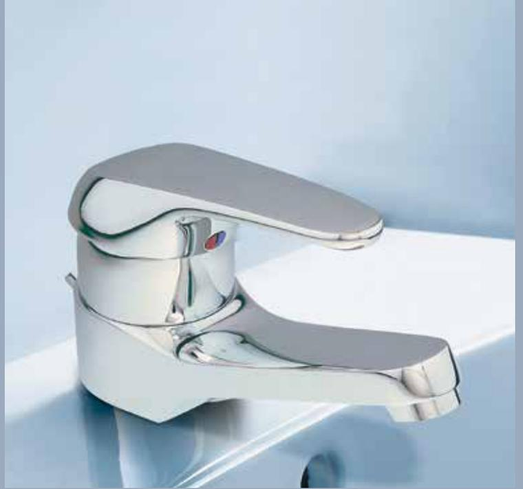
**Over-rim** single-lever, ceramic-disk, bidet fitting with cast brass body. For use on any single-hole bidet. Includes directional ball-joint & pop-up waste .
